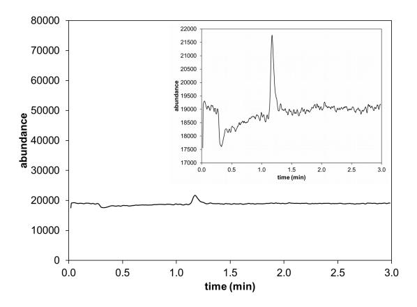
Fig. 5 HPLC-MS chromatogram of C60 sample suspended in ethanol (Redi Lion Biomedical).
