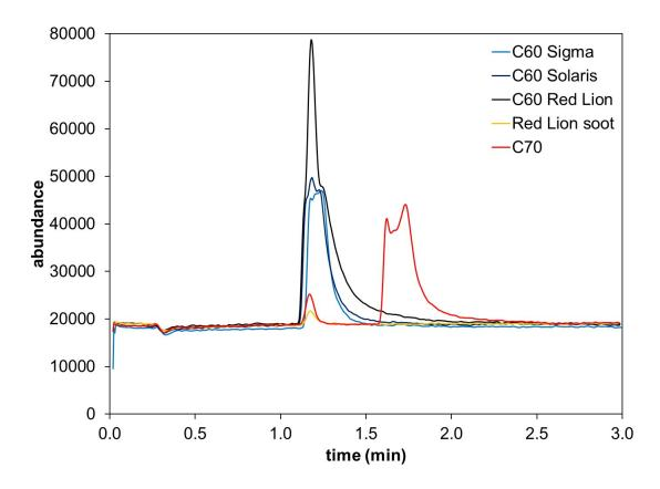
Fig. 7 Overlay of HPLC-MS chromatograms of all analysed samples.
