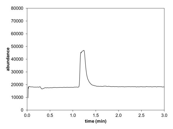
Fig. 2 HPLC-MS chromatogram of commercial C60 sample (Sigma Aldrich).
