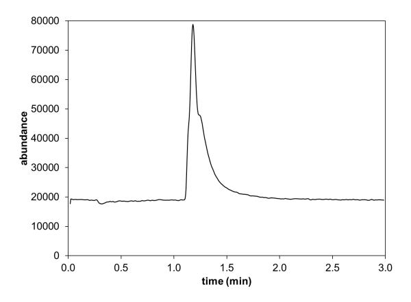
Fig. 4 HPLC-MS chromatogram of C60 sample suspended in ethanol (Red Lion Biomedical).
