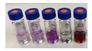
Fig. 1 From left to right: commercial sample of C60 (Sigma Aldrich), commercial sample of C60 (Solaris Chem), C60 suspended in ethanol (Red Lion Biomedical), C60 soot suspended in ethanol (Red Lion Biomedical) and commercial sample of C70 (Solaris Chem).
