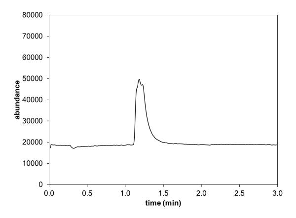
Fig. 3 HPLC-MS chromatogram of commercial C60 sample (Solaris Chem).
